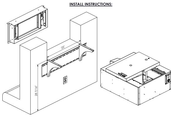
STEP 1: WITH UNIT SLIGHTLY OPEN REMOVE 8 MOUNTING SCREW FROM INSIDE OF UNIT HOLDING ON THE FRONT FASCIA AND CAREFULLY REMOVE FASICA AS WIRES WILL COME WITH IT AND SET ASIDE FOR LATER.
