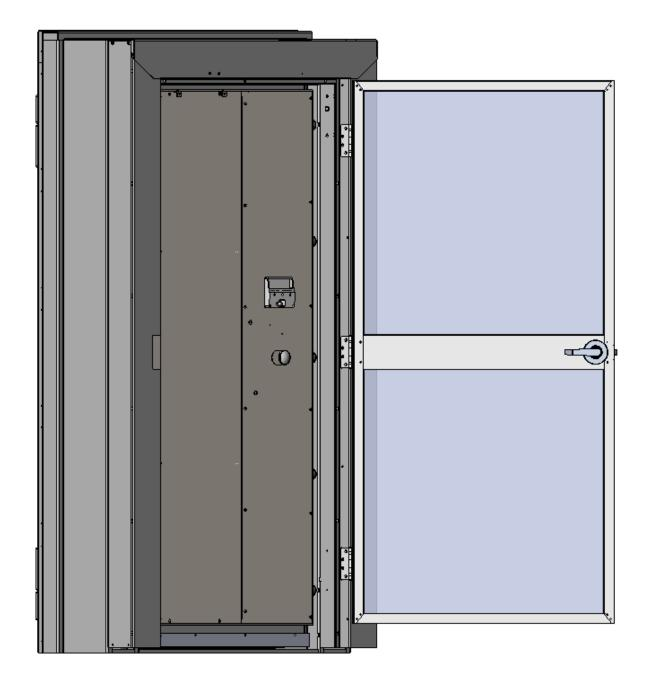
Use the provided flat head screws to fasten the hinges to the back frame.
