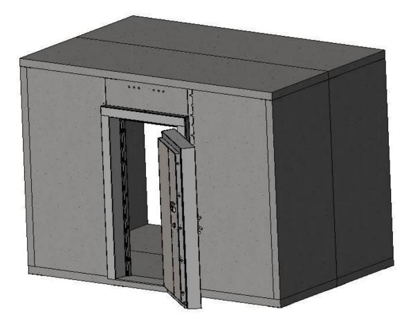
The door is now ready to open. If door swing is acceptable the door still **must be welded on inside of the vault** to match outside. Factory recommends **at least 3" long welds** top, bottom, and middle on the inside and outside. (If necessary, use provided 12" angles to bridge the gap while welding the inside)
