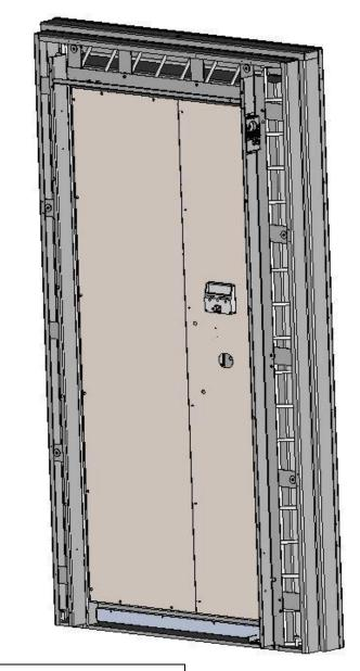
Using the 3/8 bolts provided fasten the inner left, the inner right, and the inner top.
