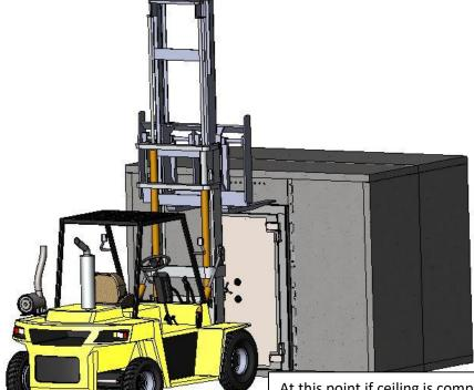
At this point if ceiling is complete, one installer must remain inside the vault to remove the bolts for the door retainer. (Note: If possible, leave one ceiling panel off to allow enough light in for final welding and allow you to pass tools back and forth.
