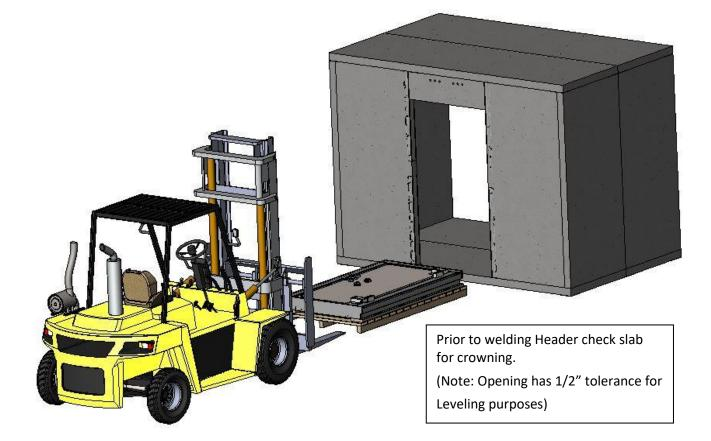
Hyde Park Vault door is shipped Face up in the crate Verify opening is plumb, level, and square (Jambs and Header should be coplanar). Verify opening is 50" x 85 5/8". (Note: Ceiling panels are to be installed flush the edge of the wall panels)
