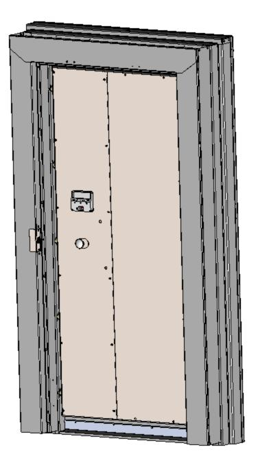
Using the  $10-32 \times 1/2$  screws provided fasten the outer top trim. The outer top trim sits on the outside of the previous installed parts.
