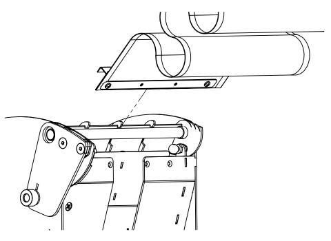
Step #3 Test operation of hopper with flex chute installed.
