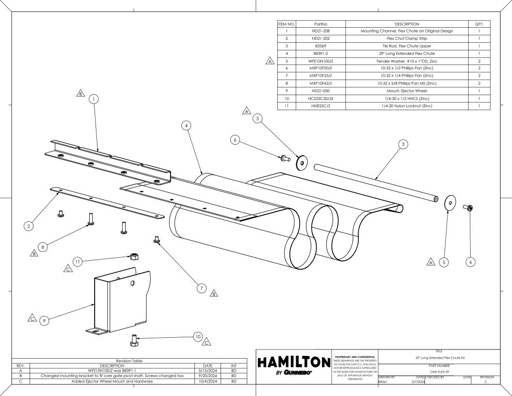
Step #1 With two center screws loosened or removed, insert flex chute mounting bracket (ND21-208) over gate pivot shaft as shown.
