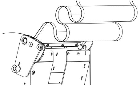
Step #2 Apply thread locker to two 10-32 x 5/8 screws. Tighten screws securing bracket to gate pivot shaft and flex chute to bracket.
