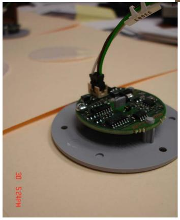
Photo cell plugs into the TX panel (transmit) the cable attached to the photo cell may or may not be used. When the cable is not required you simply unplug from the photo cell and plug the photo cell directly into the TX panel.
