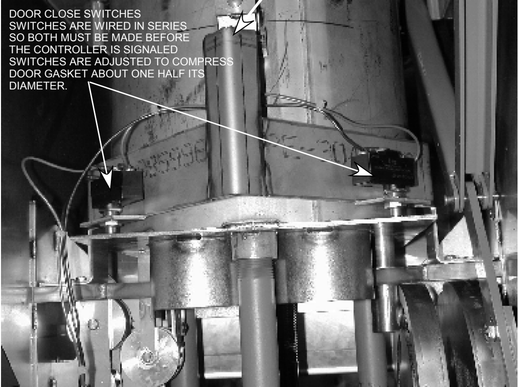
DOOR CLOSED AND CARRIER ARRIVAL SWITCHES
