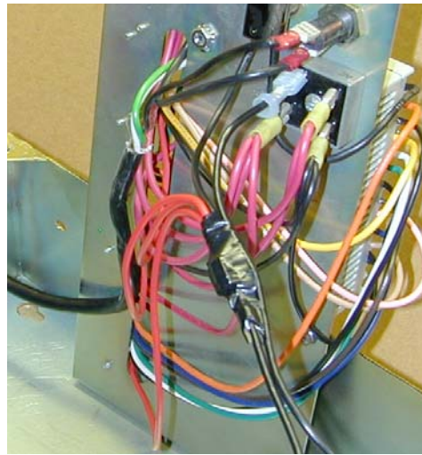
Step#7 Insulate the connection made in step #5.
