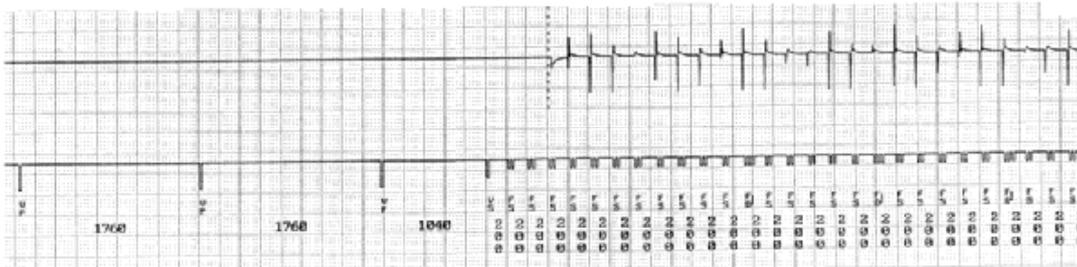
Stimulation test during exposure. At the left side (before stimulation) the ICD is pacing properly. After set-in of the stimulation the ICD detected the fibrillation correctly.
