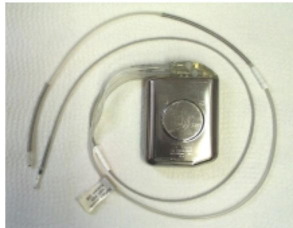
**Figure 19:** The two-chamber ICD model 'GEM DR 7271' (Medtronic)
