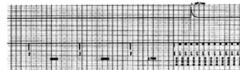
Cut-out of the stimulation test during exposure. At the left side (before stimulation) the ICD is pacing properly. After set-in of the stimulation the ICD detected the fibrillation correctly.
