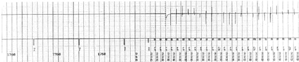
Cut-out of the stimulation test during exposure. At the left side (before stimulation) the ICD is pacing properly. After set-in of the stimulation the ICD detected the fibrillation correctly.
