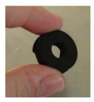
**Step#5** Remove clear differential valve disc from spindle.
