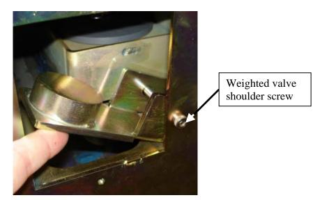
**Note:** Some previous turbines may have a stainless steel plate that is trapped behind this weighted valve installed from the factory. This plate can remain in turbine or be removed. Make sure that this plate does not cause the valve to stick or bind in its operation.
