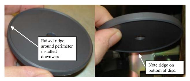
**Step#7** Install rubber washer and hairpin clip, as removed in previous steps.
