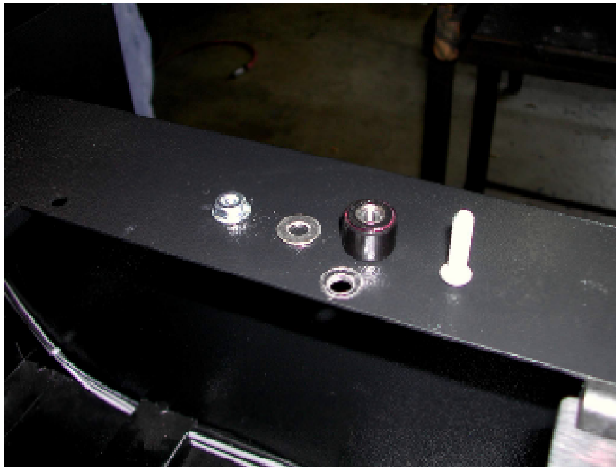
Model 400DD Deal Drawer Showing Part Number B4597 Inside Lid Cam Roll bearing Assembly
