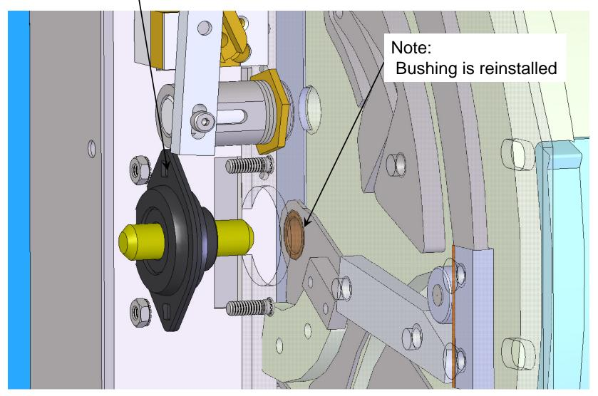
• Reinsert bearing opposite from the way it came out bearing collar toward bushing Note: Pin set screws should already be tight before reinserting
