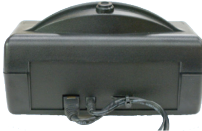
Rear of 5571 showing Cat 5 cable w/power
