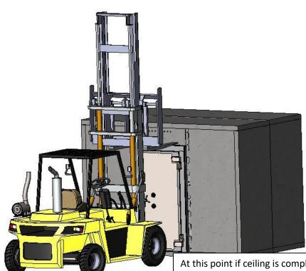
At this point if ceiling is complete, one installer must remain inside the vault to remove the bolts for the door retainer. (Note: If possible, leave one ceiling panel off to allow enough light in for final welding and allow you to pass tools back and forth.
