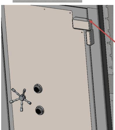
Raise the door up by adjusting the set screws on the top and bottom hinges. Get the door square before welding it in place.
