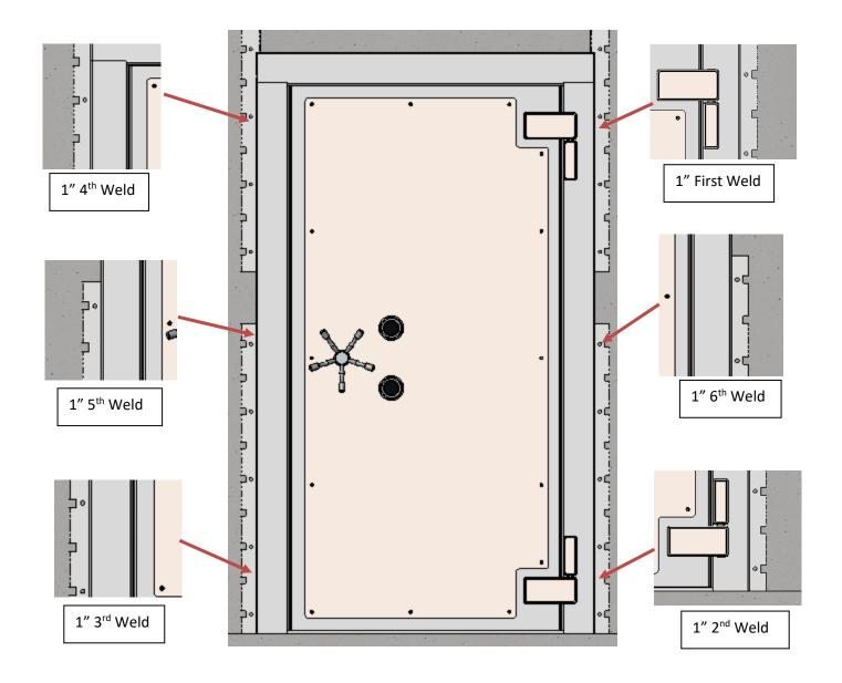
IMPORTANT!! A MINIMUM OF (6) 1" WELDS MUST BE COMPLETE BEFORE OPENING THE DOOR!!!
