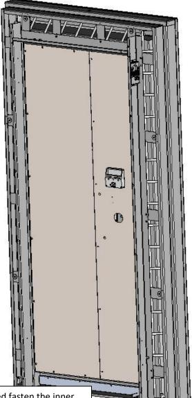
Note the position of the heat sensor. It should be installed on the strike side with the sensor lining up with the locking bolts. There is a circle knockout which will locate the heat sensor. It should be fastened with 2 8-32 screws and 2 KEPS nuts which are included in the hardware kit.
