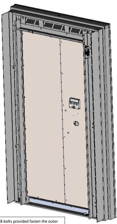
Using the 3/8 bolts provided fasten the outer left side and the outer right side
