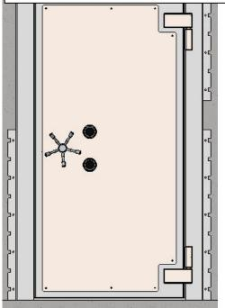
Once you have leveled and shimmed the door and all is acceptable, it is time to weld in place. Start by putting a 1" long weld in six places before opening the door.
