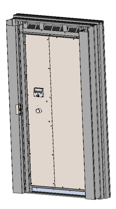
Using the  $10-32 \times 1/2$  screws provided fasten the vertical rear strike extension and the vertical rear hinge extension. Both parts sit on the outside of the previously installed parts.
