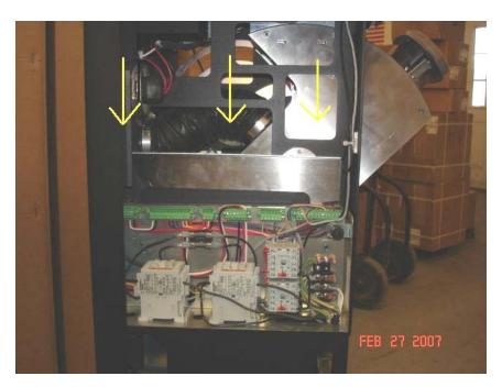
**STEP 4:** Align the mounting holes in the stainless steel bracket, the control panel, and the HA47 frame and re-install two mounting screws.
