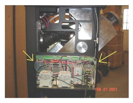
STEP 3: Insert stainless steel bracket B6949 down between the control panel and frame.
