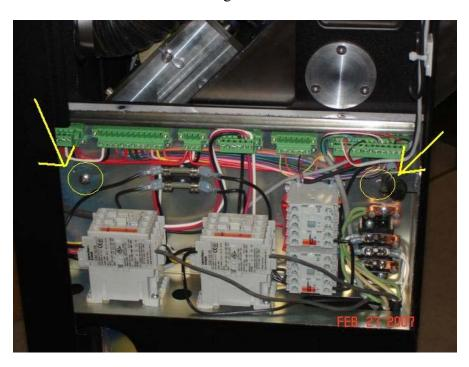
**STEP 5:** Using two, 10-32 screws, attach the cover B6948 to the holes in the bracket B6949. The cover B6948 has nock-outs to allow wires to be routed through. Seal around wires if these knock-outs are removed..
