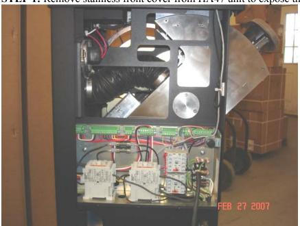
**STEP 2:** Remove two, 10-32 screws, mounting the control panel to the frame.
