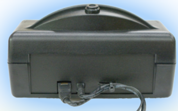
Rear of 5571 showing Cat 5 cable w/power
