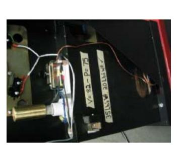
Uncoil thermostat tube and position thermostat along side the turbine box as shown. Set thermostat control to 40 degrees.
