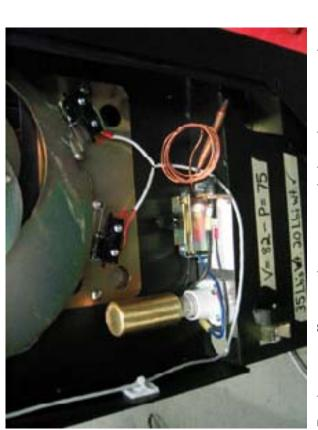
Peal paper off mounting tape and place heater as shown Dress existing wires away from heater element
