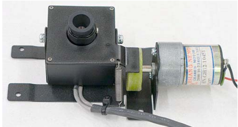
Completed Tilt Assembly
