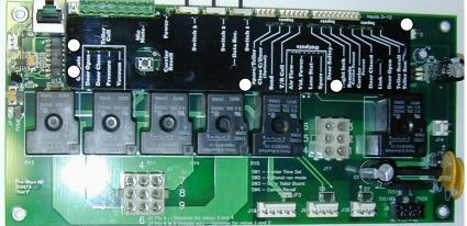
3) Using a chip puller, chip removal tool, or small prying device, pull the Prom chip straight from its socket attached to the circuit board. (Care must be taken when removing Prom Chips from the control board socket to prevent damage to the socket or control board. Damaging the socket or control board can cause the unit to fail or have unexpected behaviors.)
