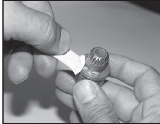
Figure 23 - Apply Lubricant to Hub
