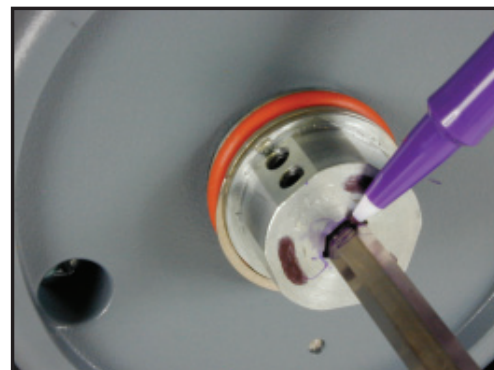
Figure 21 - Mark Spindle Flush to Hub
