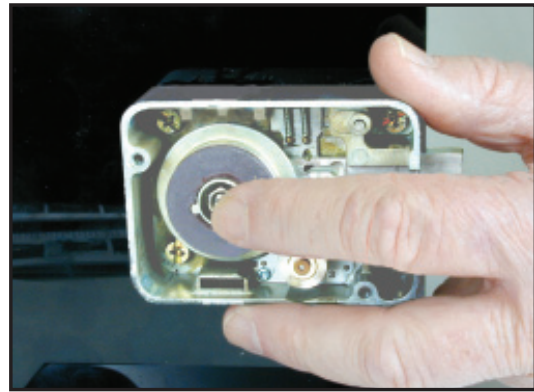
Figure 25 - Maintain Pressure on Spindle Assembly
