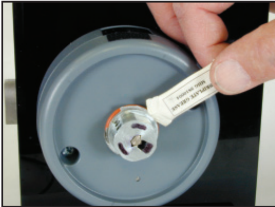
Figure 27 - Apply Lubricant to Ret. Ring
