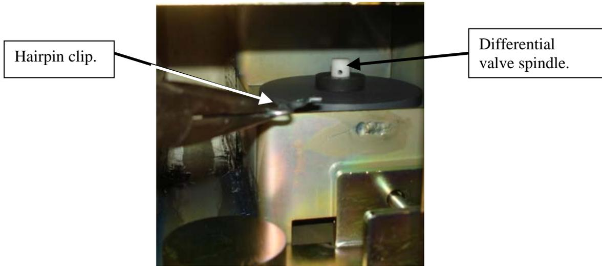
**Step#4** Remove rubber washer from differential valve spindle.
