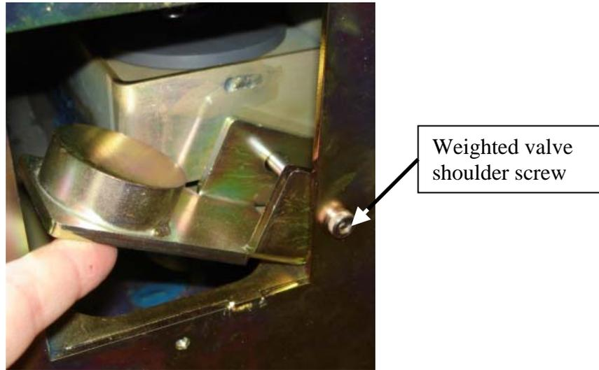
**Note:** Some previous turbines may have a stainless steel plate that is trapped behind this weighted valve installed from the factory. This plate can remain in turbine or be removed. Make sure that this plate does not cause the valve to stick or bind in its operation.
