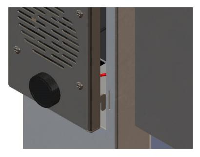
2. Align Tabs of Ventilator Face to Slots in Frame Stainless Steel. Insert into slots then carefully slide Ventilator Face downward until it bottoms out in slot of Frame Stainless Steel.
