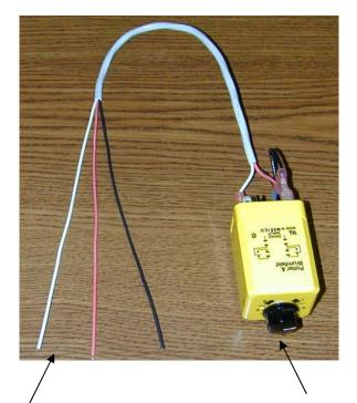
Field Connections Black - #2 Terminal on Counter Teller White - #20 Terminal on Counter Teller Red - #8 Terminal on IRT5000 Control Unit **Timer Setting** Set timer to the #1 mark. Make sure this time is less than turbine run time.
