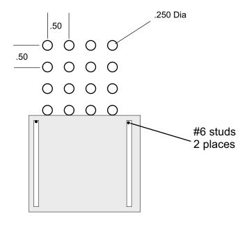
Holes in top of Downsend Turbines with slide plate to Adjust air flow.
