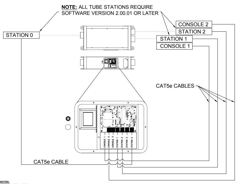
TYPICAL INSTALLATION STATION 0 = CUSTOMER UNIT STATION 1 = TELLER STATION 1 STATION 2 = TELLER STATION 2 ALL STATIONS MUST HAVE I/O CONTROL BOARDS
