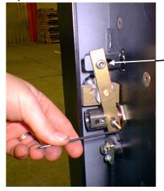
**Do Not** loosen or remove the shoulder screw in the top of the lock pin actuator.
