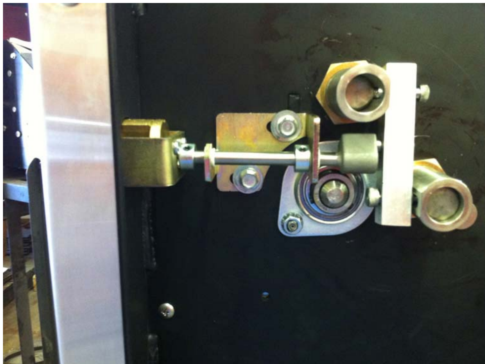
VIEW OF SPACER AFTER INSTALLATION (SPACER WILL NOT ALLOW BRONZE BUSHING TO WORK OUT OF BUCKET)
