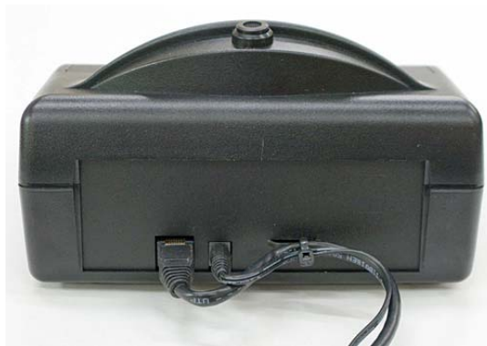
Rear of 5571 (with Cat 5 cable & power supply connected)
