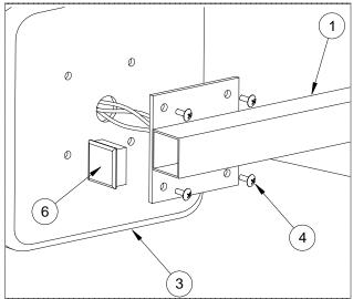
Step#3 Apply a small amount of silicone sealant to the mounting plate on the mounting arm (#1) to seal between TTV unit (#3) and plate.
