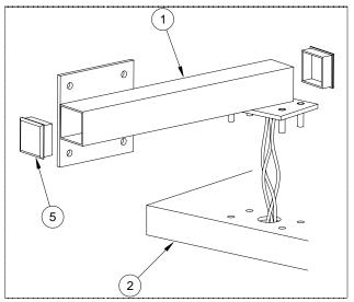
Step#2 Apply a small amount of silicone sealant to the bottom of the plate on the mounting arm (#1) to seal between customer unit and plate.
