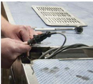
Front wiring harness connectors
